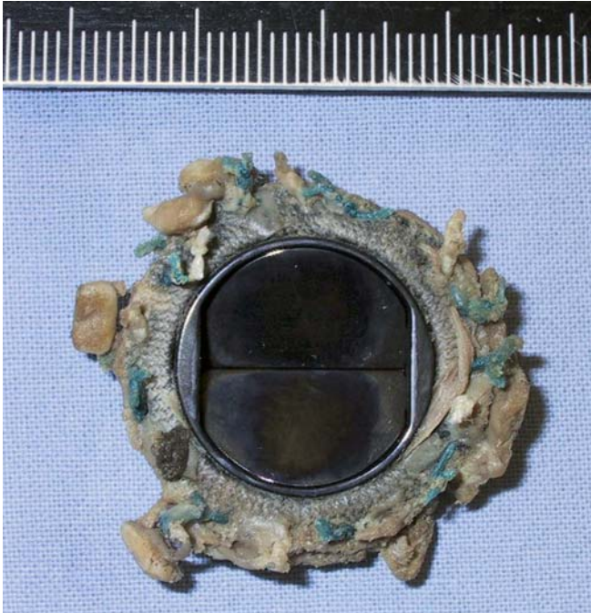
Fig. 1 Completely detached aortic valve prosthesis found in the ascending aorta. Note the remains of sutures and the nearly circular aortic particles. The two lightest patches are used as abutments when suturing the valve in the implantation site
